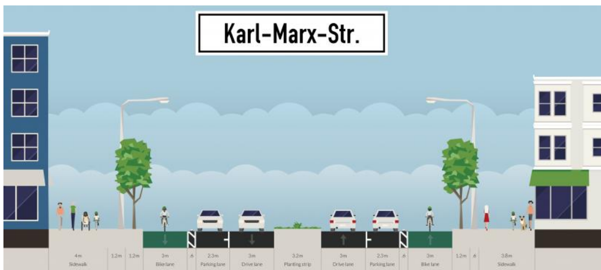
Figure 25 - Cross-section of suggestion for a temporary protected bike lane on Karl-Marx-Straße (Netzwerk fahrradfreundliches Neukölln 2017)
