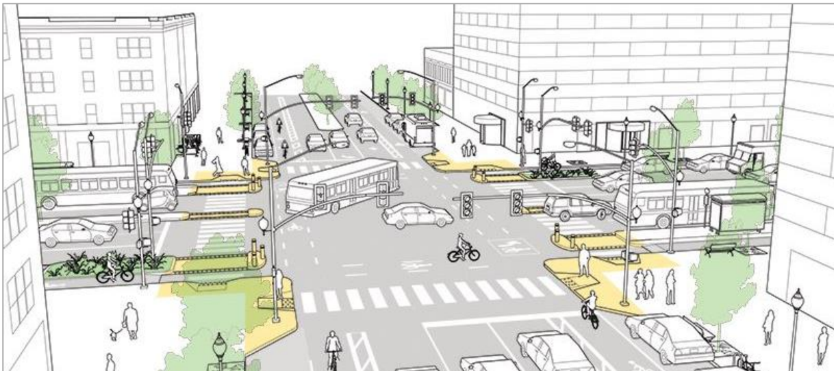
Figure 23 - Major intersection, protected design (NACTO 2013)
